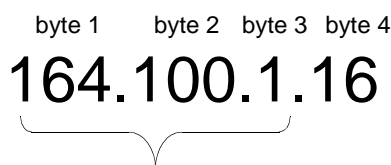
FIGURE 3-6 Determining the Net Portion of the IP Address the Customer Uses for the System Center
