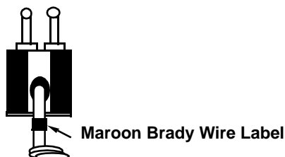
FIGURE 8-18 Identifying Tradenet and Tradenet MX Handsets
